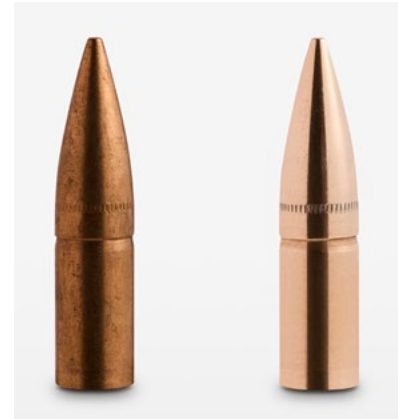
A projectile before (left) and after (right) the finishing treatment in the circular vibrator.
