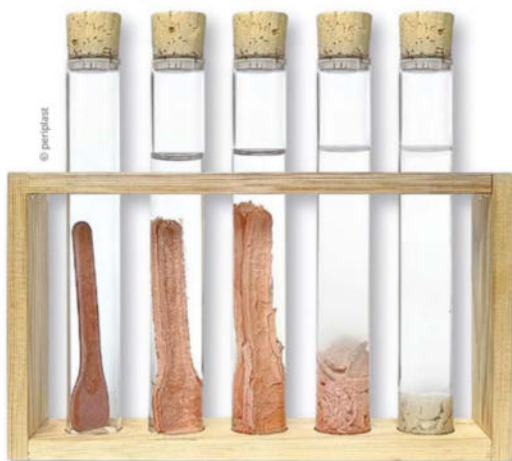
If exposed to water, after six weeks the spoons are nearly completely dissolved.
