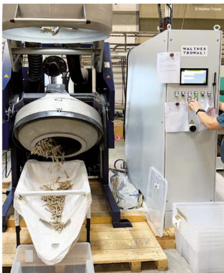
Coated ice cream spoons are discharged from the Rotamat system.
