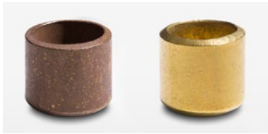
Cups before (left) and after (right) the treatment in the circular vibrator
