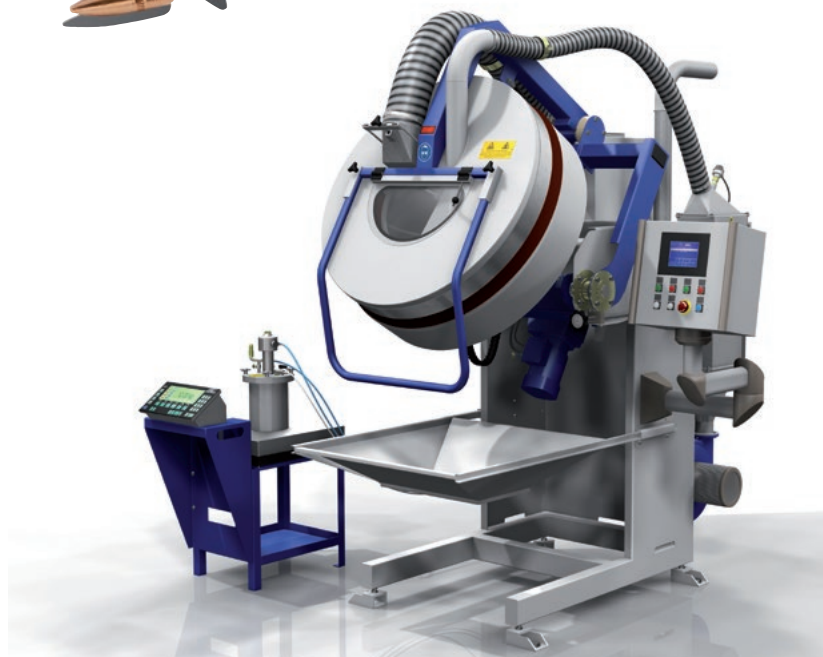
The Rotamat coats projectiles with a lubricant finish.
