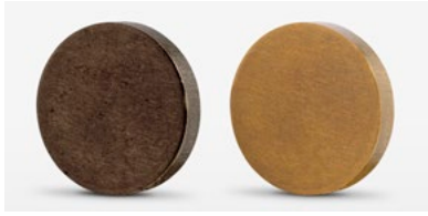
Round blanks before (left) and after (right) washing in the circular vibrator
